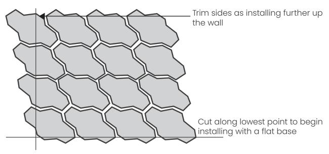
**Installing with Dry Joint:** Take time once the pattern is laid to cut thin stones to fill small gaps between the larger joints. This is very important, it will break up the pattern and provide the perfect hand crafted stone masonry look.
