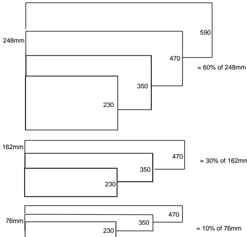
Sample Installation pattern – like brick work, avoid straight vertical lines when applying the stone
